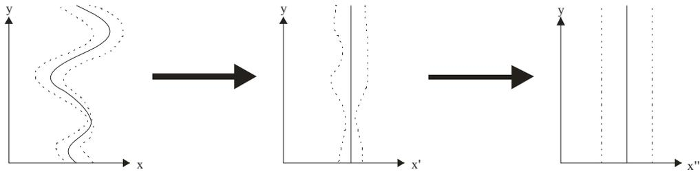
**Figure 3:** Stratigraphic coordinate transformation in plan. First the curvilinear features are removed, followed by standardizing the thickness of the channel (after Deutsch 2002).
