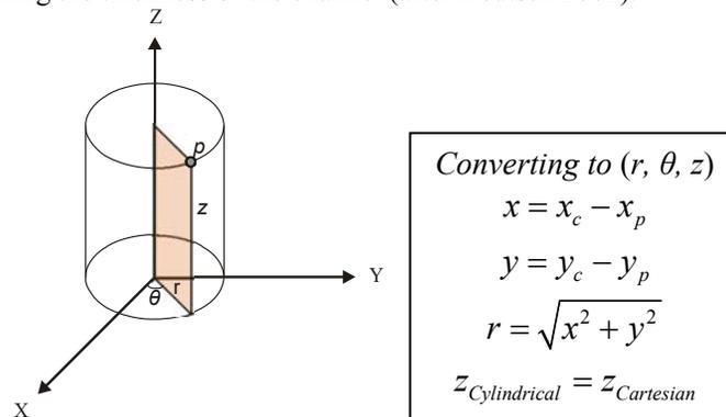
**Figure 4:** Defining a point in space ( $p$ ) using cylindrical coordinates ( $r$ ,  $\theta$ ,  $z$ ).
