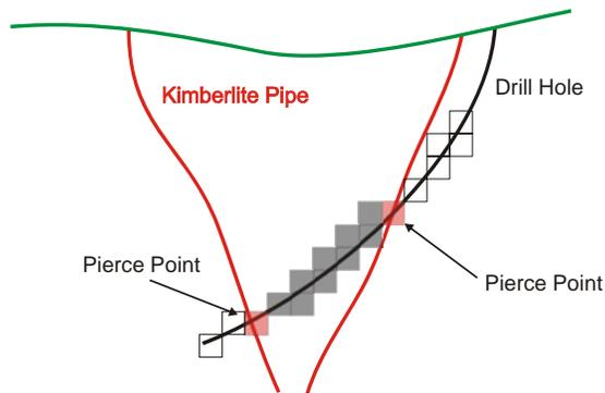
**Figure 12:** It is known that the white blocks are outside the pipe and the gray blocks must be kimberlite.
